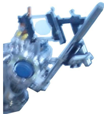
Lens holder with alignment stage and rod included in Optical component for laser beam introduction
