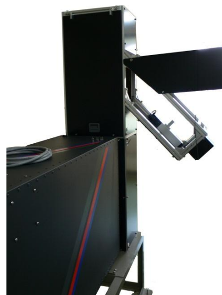
Excimer laser stand and laser optics with protection hood mounting CompexPro 102 Excimer Laser
